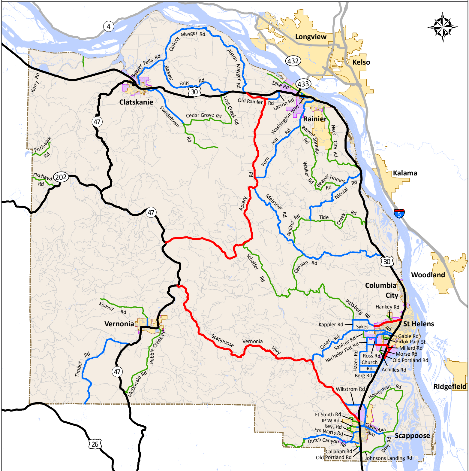
Figure I - Roadway Functional Classification
